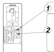
Press the FUNCTION selector so that the display indicates  $\Re$  (COOL).
