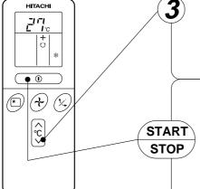
Press the ① (START/STOP) button. Cooling operation starts with a beep. Press the button again to stop operation. The cooling function does not start if the temperature setting is higher than the current room temperature (even though the ① (OPERATION) lamp lights). The cooling function will start as soon as you set the temperature below the current room temperature.
